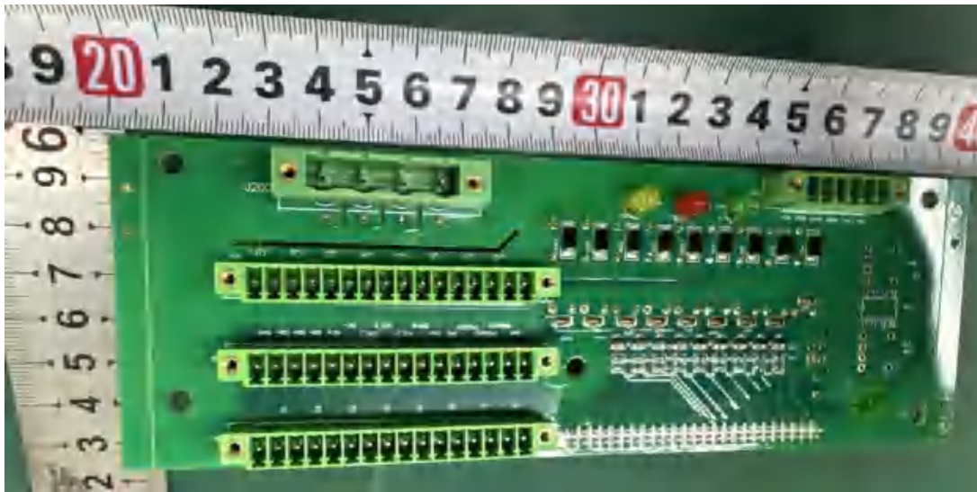
Figure 29 component side of terminal board
