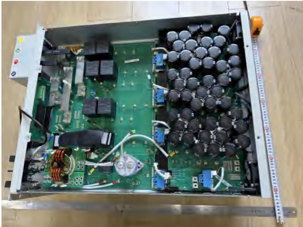
Figure 9 Inside view without control board, isolation board
