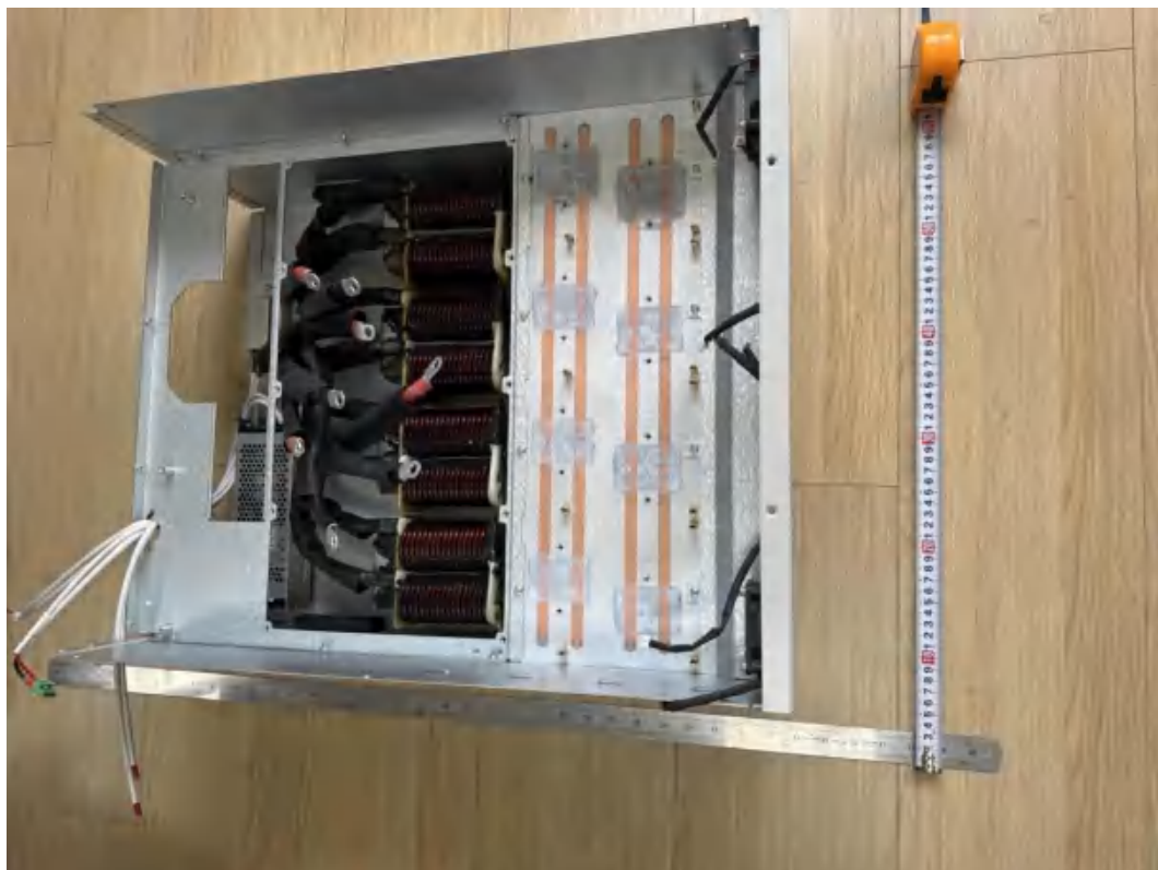
Figure 12 Inside view of enclosure without PCBs
