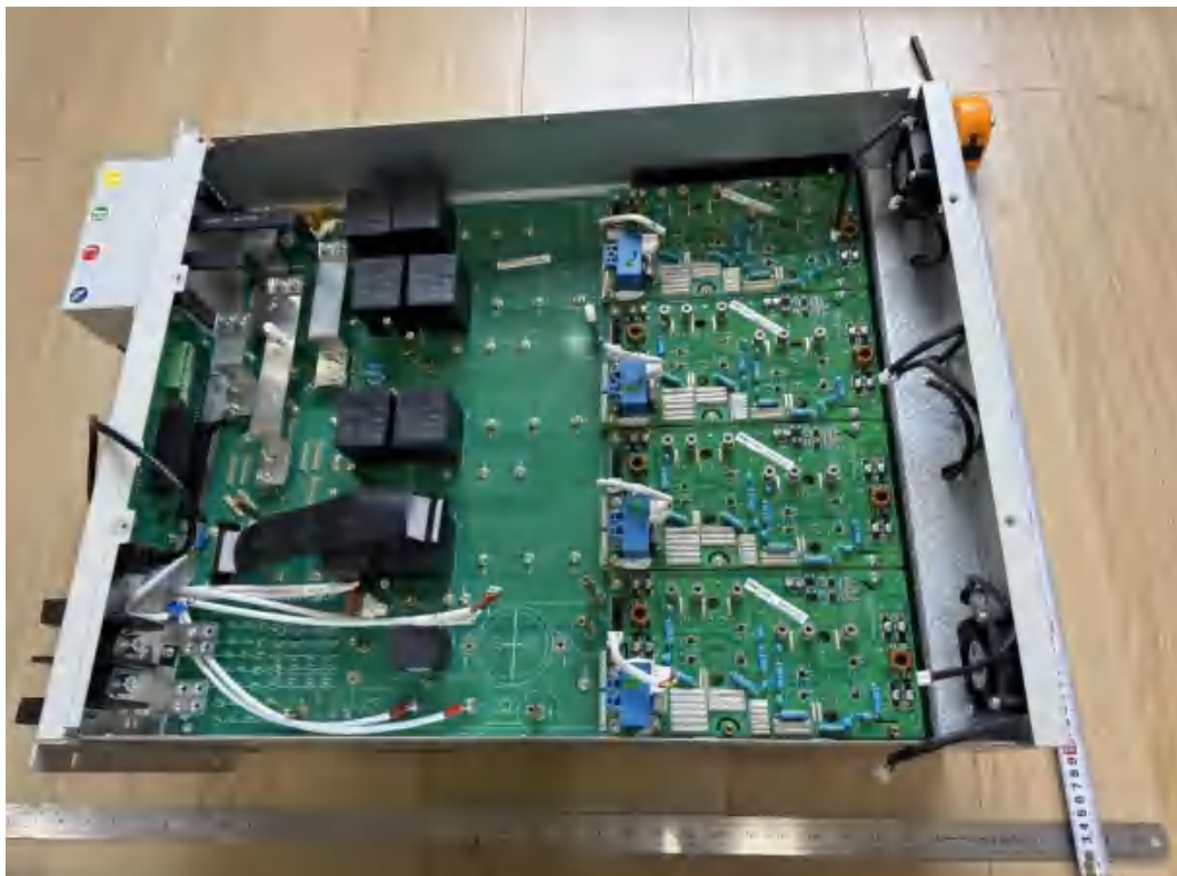
Figure 10 Inside view without control board, isolation board, Capacitor board, and DC filter board
