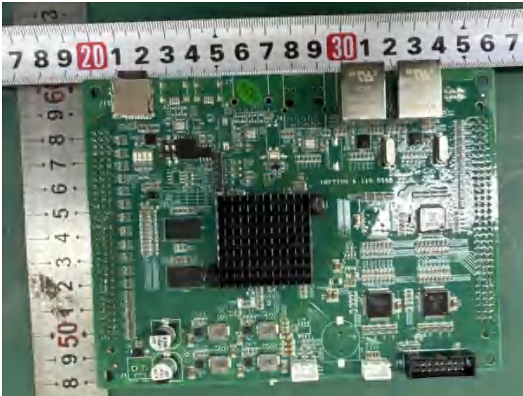
Figure 13 component side of core board
