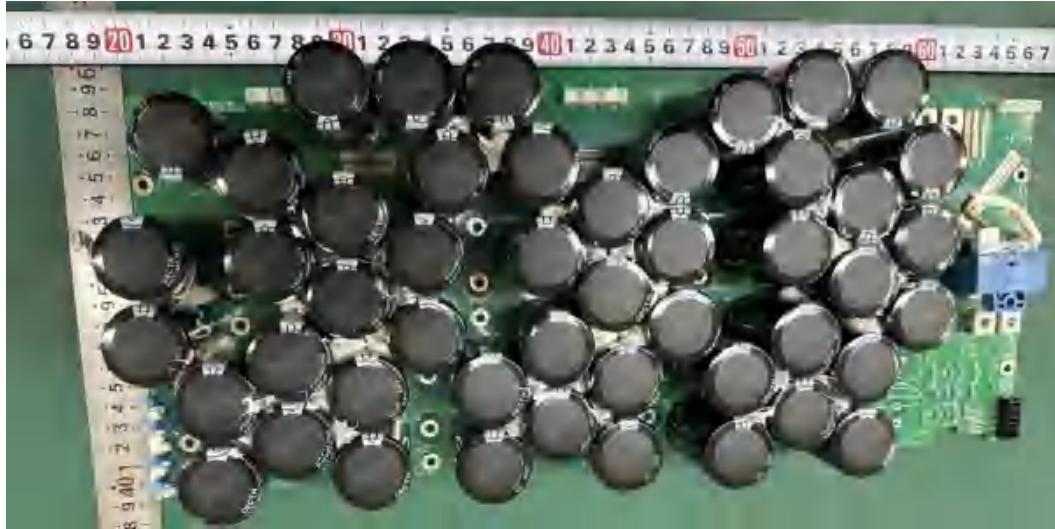
Figure 21 component side of capacitor board
