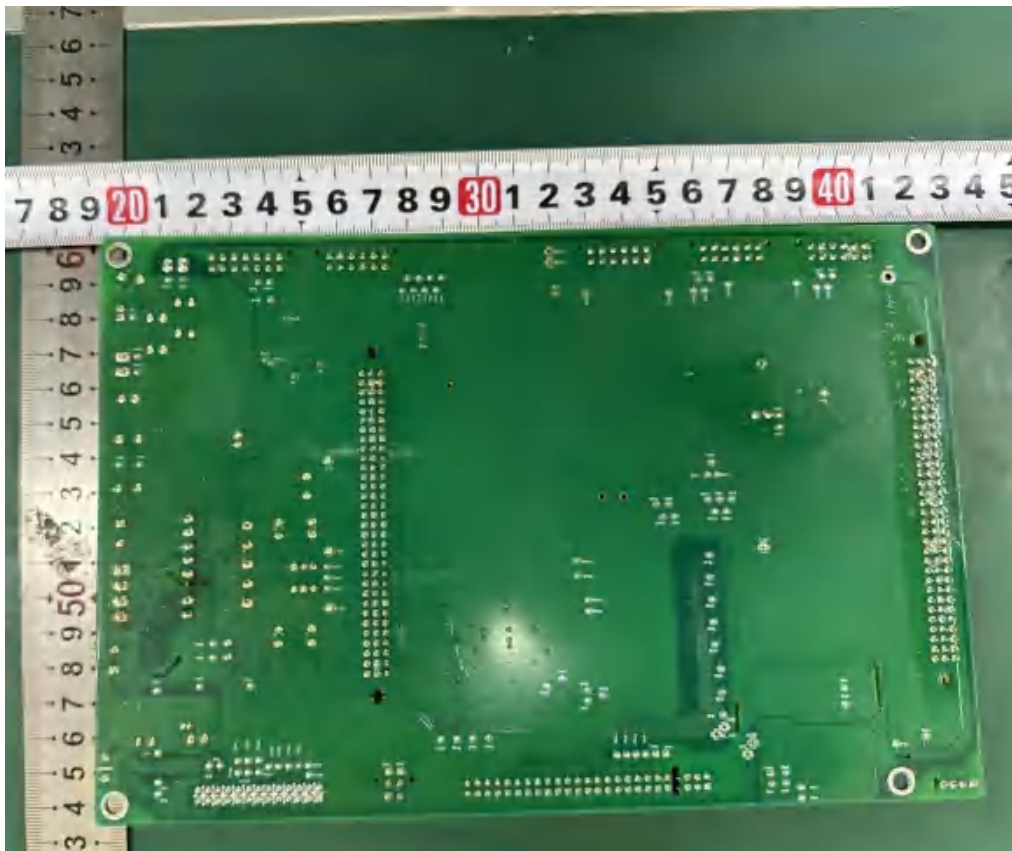
Figure 16 trace side of control board
