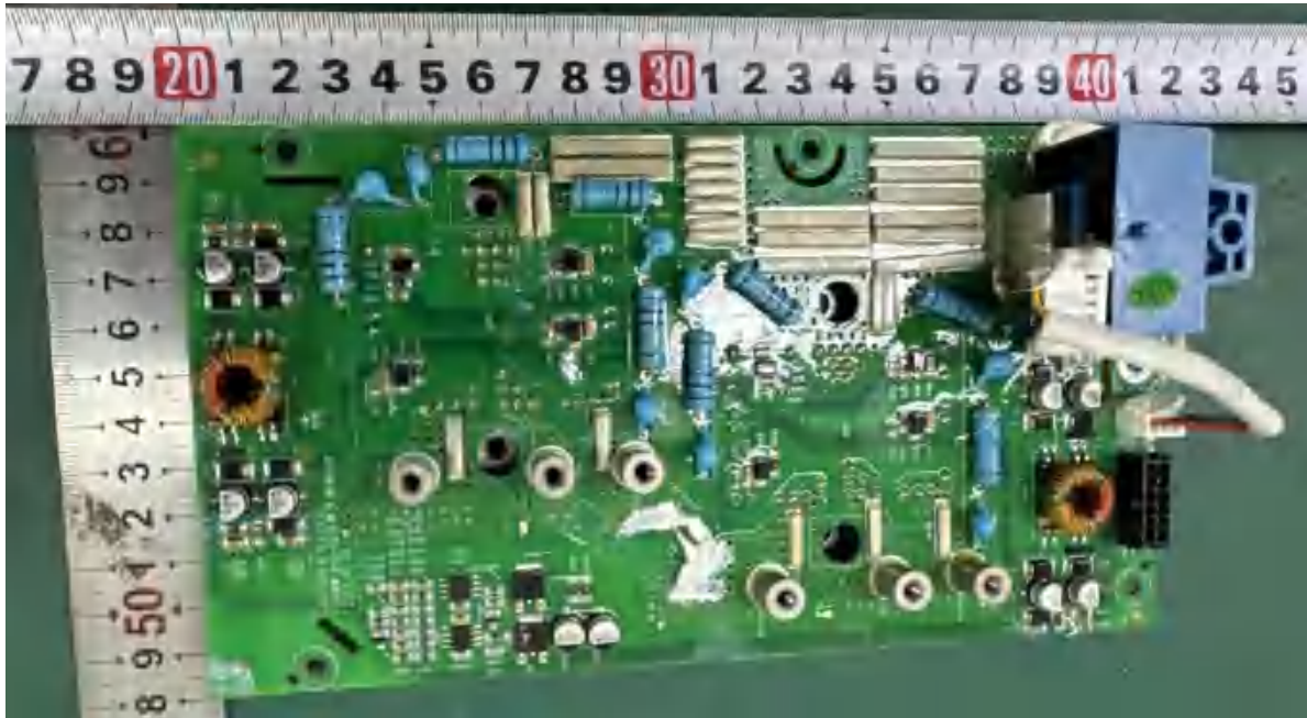
Figure 23 component side of power board
